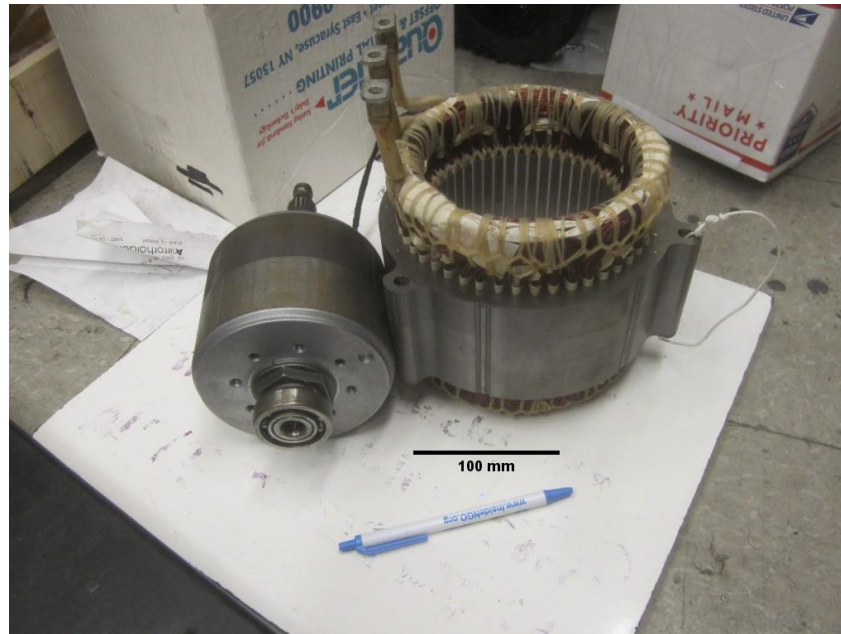
Figure 2: Mercury Milan Hybrid MG1 rotor (left) and stator (right)
