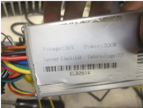
Figure 23: 500W electric bicycle controller
