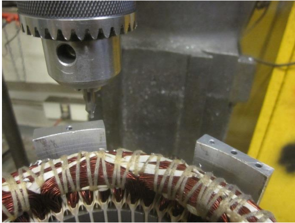
Figure 17: drilling holes for back plate mounting Figure 18: completed front bearing bore
