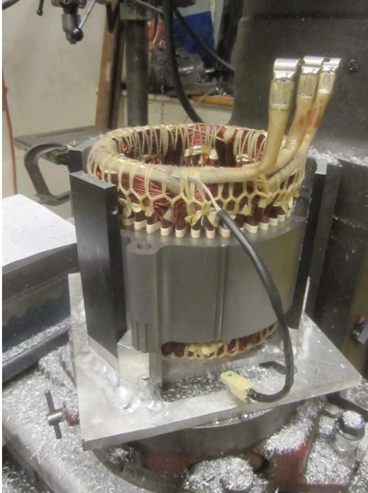
Figure 16: Preparing to machine lower bearing bore
