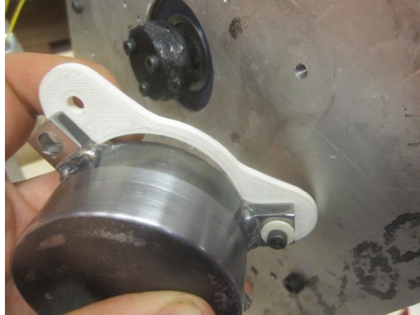
Figure 47: printed ABS spacers for electrical isolation of the sensor housing
