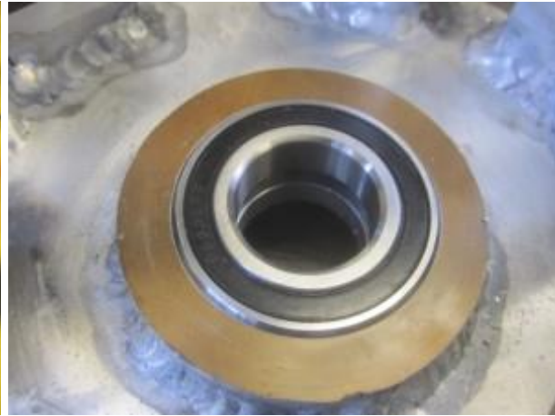
Figure 17: drilling holes for back plate mounting Figure 18: completed front bearing bore
