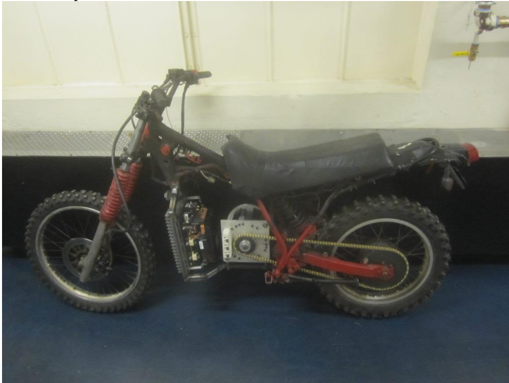
Figure 54: Motor and inverter attached to frame
