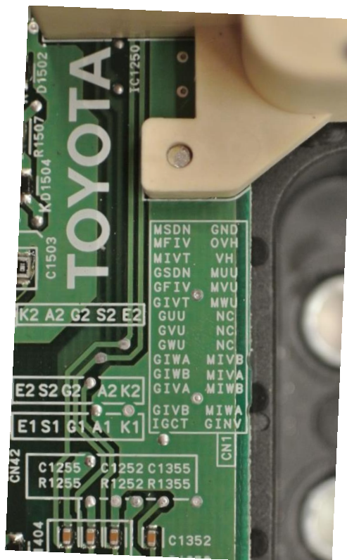
Figure 30: Inverter module pinout printed on circuit board
