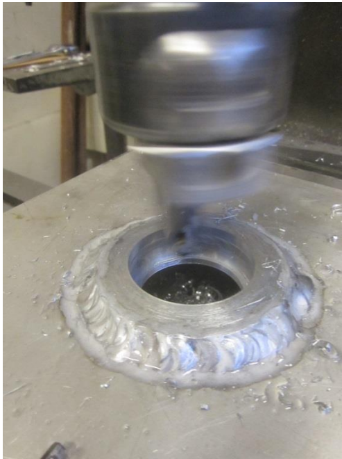
Figure 21: rear bearing housing boring
