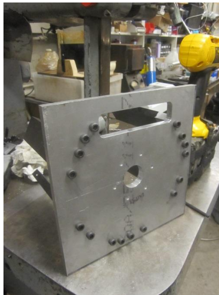
Figure 11: unbored motor housing, top view Figure 12: unbored motor housing, bottom view
