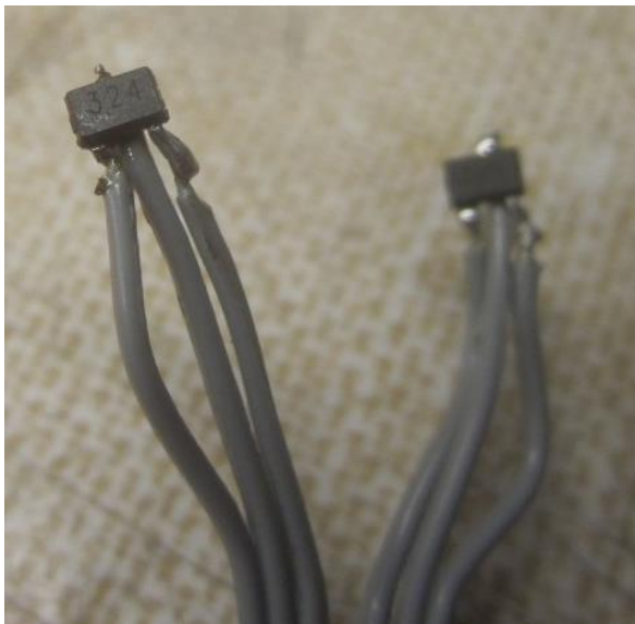
Figure 37: Allegro A1324 analog hall sensors Figure 38: analog and digital hall sensor spacing
